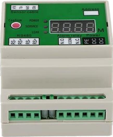
AG-LLM1 Location water leak controller can detect 1500m sensing cable. It'll alarm by flash and sound once there's water leaks on the cable, and the leakage point will display on the LCD screen and the relays will be on automatically.
