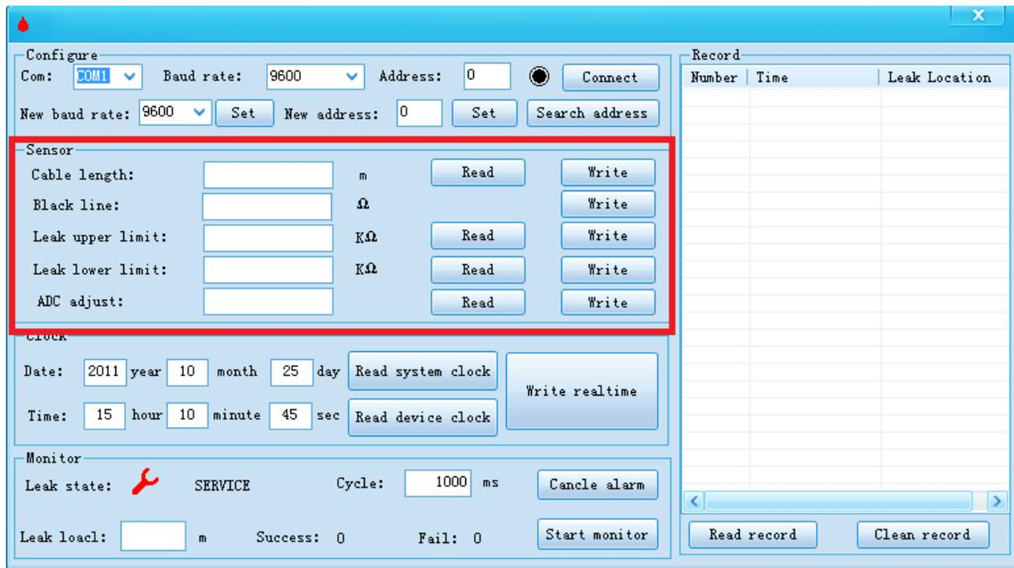
The screenshot shows the configuration window for the AG-LLM1 device. The 'Sensor' section is highlighted with a red border. It includes the following fields and buttons:
